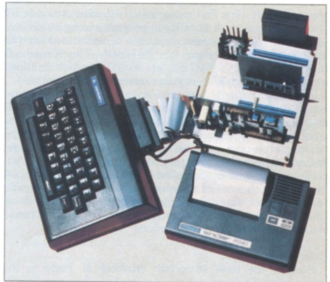
Photo 1. Instrumentation set-up. ZX81 with Suntronics KB conversion, TS2040 printer, 16K RAM, Computer Continuum 8 channel A/D D/A Board, CC expansion board (shielded) and "special purpose" RAM/function board. Not shown dual Basic/Forth operating systems.
